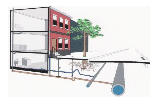
The **brown pipe** connecting the house to the sewer in the street is the house sewer lateral. The **blue pipe** connecting the house to the street is the house water service. Note that the sewer lateral is approximately six feet below the sidewalk and that the roots of the tree are approximately two feet below the sidewalk.
